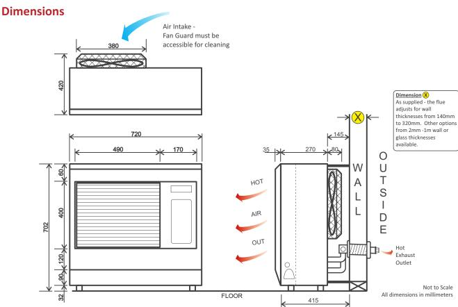
Unpacked Weight: 40kg - Packed Weight: 46kg - Packed Size: 785mm x 760mm x 500mm
